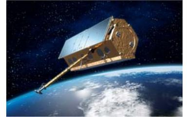
Fig. 2: Artist view of the TerraSAR-X satellite showing the X-band radar antenna (towards the sun) and the downlink antenna (at a 3 m long boom).
