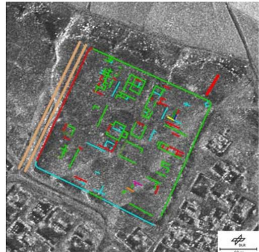
Fig. 6: TerraSAR-X image. High-resolution Spotlight mode with experimental 300 MHz bandwidth; spatial resolution: 1 m; polarization: horizontal; inclination angle: 34.87°; stacking of nine data takes; time of data take: February - May 2012 (© DLR, 2012).
