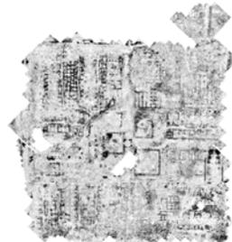
Fig. 3: GPR depth slice between 20 and 30 cm depth. GSSI SIR-3000 with 400 MHz antenna; Sensor&Software Noggin with 500 MHz antenna; PulseEKKO 1000 with 900 MHz antenna. Sample density: 5 x 25 or 50 cm.
